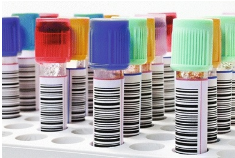
FIGURE 7.4 Sample collection tubes are identified with bar code labels. (Photograph courtesy of Siemens.)
